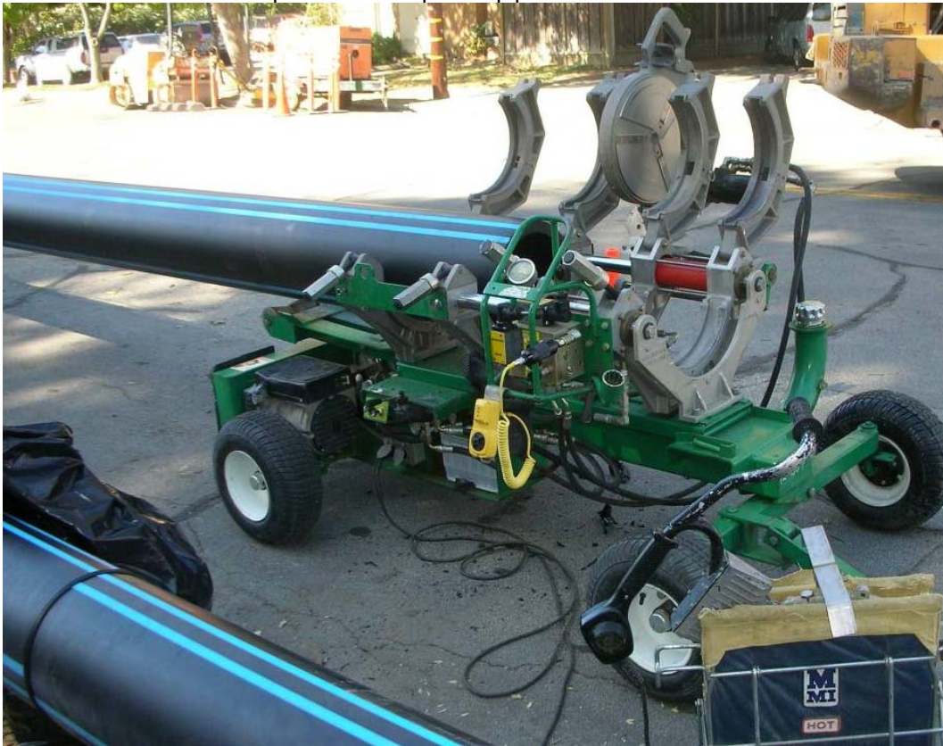
Figure 3. McElroy Fusion Machine.
