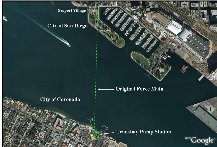
Figure 1: Aerial Photo Showing Approximate Alignment of Original Force Main (Photo Courtesy of Google Earth)
