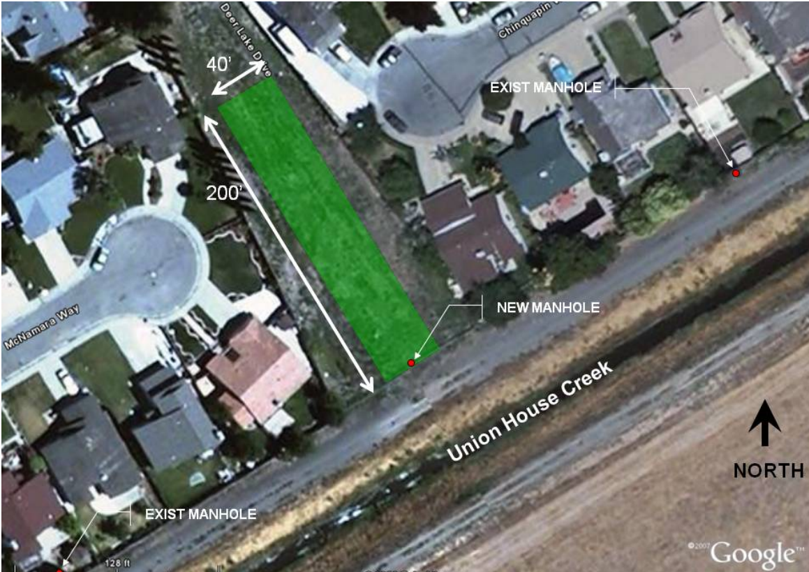
Figure 4: Installation of new manhole for installation of CIPP
