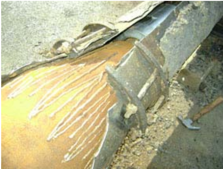
Figure 5. Above ground test, coupling successfully split.
