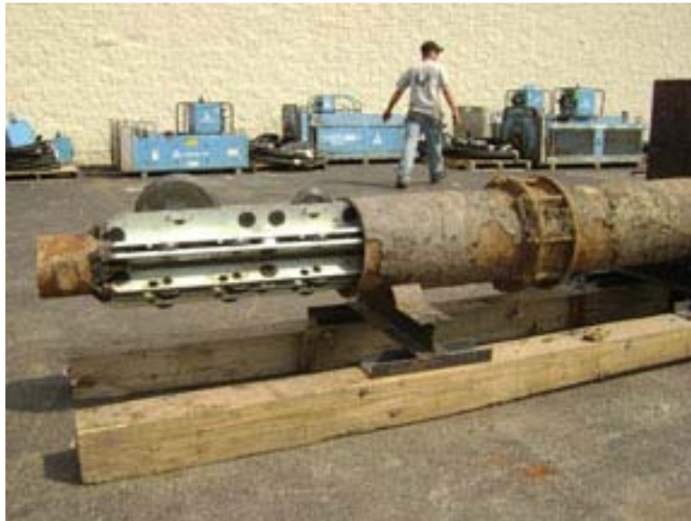
Figure 3. Above ground test, launching the cutter head.
