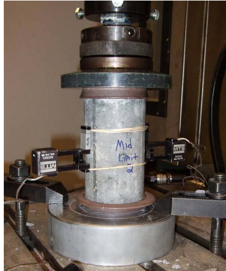
Concrete Compression Test Source: www.wikipedia.org
